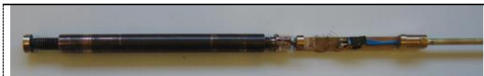
**Figure 3.** Assembled pressure cell attached to the MPMS sample rod through an adapter with a 4-pin socket mounted on it.
