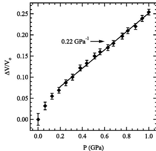
FIG. 3. Compressibility of Daphne 7373 oil. The solid line is a linear fit above 0.2 GPa.
