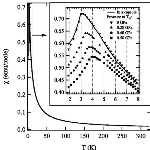
FIG. 4. Magnetic susceptibility of  $[N(C_2H_5)_4][FeCl_4]$  as a function of pressure. The inset is the zoom into the low-temperature region with the solid line showing the data collected on the sample in a standard MPMS gelatine capsule and the straw.
