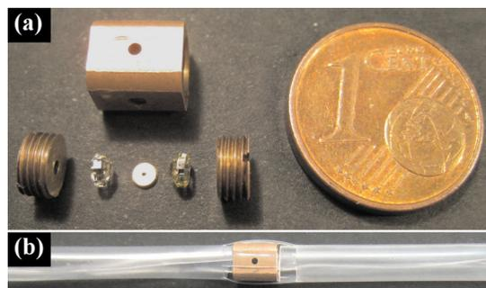
FIG. 2. (Color online) (a) Parts of the TM-DAC. (b) The assembled TM-DAC in the standard plastic straw holder of MPMS.
