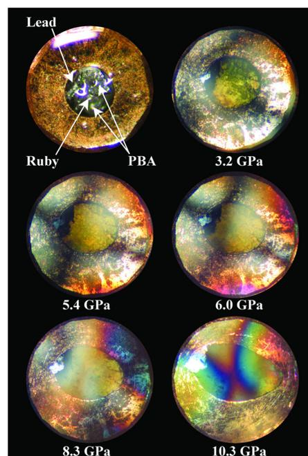
FIG. 7. (Color online) Photographs of the gasket hole taken at several pressure points during loading. The hole contains the sample of  $\text{Mn}_3[\text{Cr}(\text{CN})_6]_2 \cdot x\text{H}_2\text{O}$  PBA, a speck of Pb, and a ruby chip. The elongation of the sample hole illustrates the quality of the anvil alignment.
