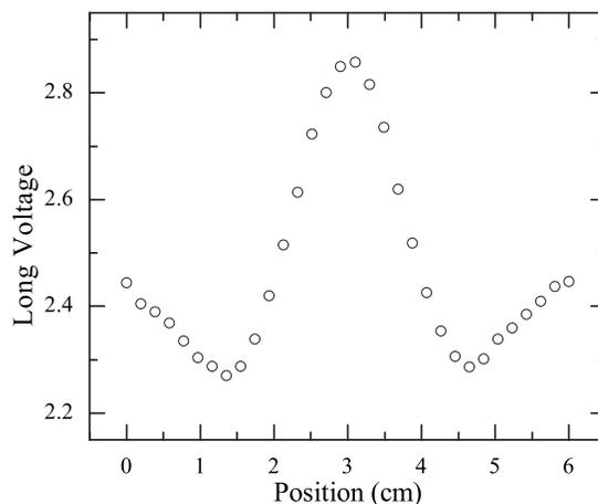
FIG. 4. Raw MPMS data generated by a scan of the empty TM-DAC over a 6 cm distance in an applied field of 20 Oe at 300 K. The resulting integrated magnetization as calculated by the MPMS software is  $1.07 \times 10^{-5}$  emu.
