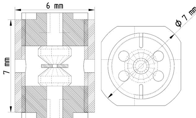
FIG. 1. Drawings of the TM-DAC with key dimensions.
