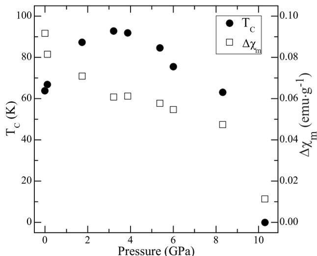
FIG. 9. The pressure-temperature magnetic phase diagram of  $\text{Mn}_3[\text{Cr}(\text{CN})_6]_2 \cdot x\text{H}_2\text{O}$ .  $\Delta\chi_m$  shows the difference between the values of mass susceptibility taken at 40 K,  $\chi_m(40 \text{ K})$ , and 120 K,  $\chi_m(120 \text{ K})$  (see Fig. 8).
