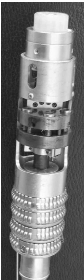
Figure 3. The pressure cell on the  $^3\text{He}$  platform.
