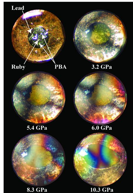
FIG. 7. (Color online) Photographs of the gasket hole taken at several pressure points during loading. The hole contains the sample of  $\text{Mn}_3[\text{Cr}(\text{CN})_6]_2 \cdot x\text{H}_2\text{O}$  PBA, a speck of Pb, and a ruby chip. The elongation of the sample hole illustrates the quality of the anvil alignment.
